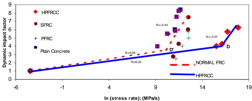
Figure 1. Stress-Rate Sensitivity of HPFRCC, Ordinary Steel Fiber Reinforced Concrete (SFRC), Ordinary Polypropylene Fiber Reinforced Concrete (PFRC) and Plain Concrete. Notice the reduced sensitivity of HPFRCC and the rightward shift of the ‘knee’.
