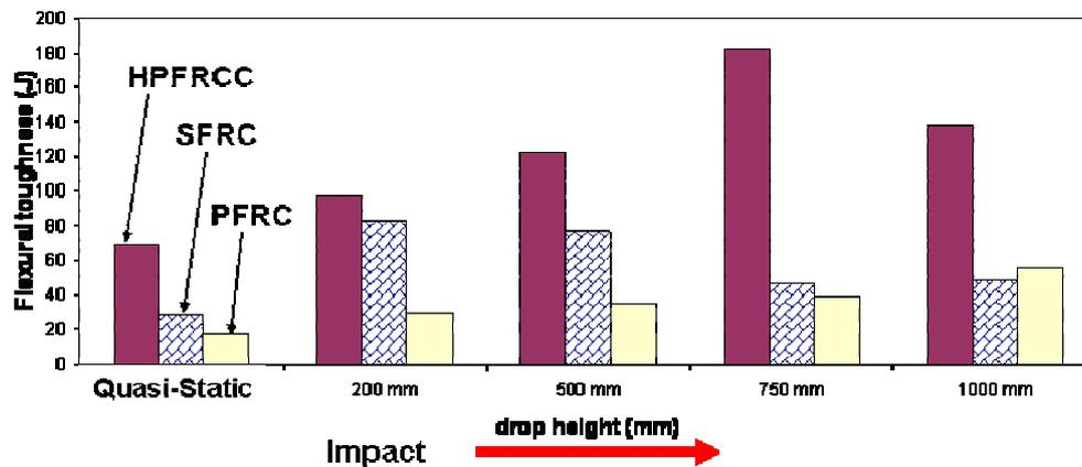
Figure 2. Reduced Toughness in FRC and HPFRCC at High Strain-Rates
